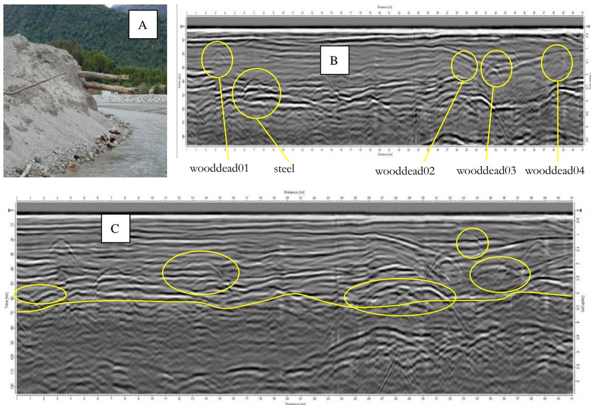
**Figure 1:** Buried dead wood exposed by channel reworking and bank erosion (A); radargram of the survey showing the buried dead wood (B), and the complete radargram (C).
